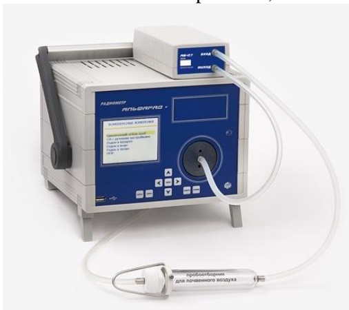
Fig. 1. Alfarad plus device for the determination of radon in air and water
