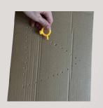
2. To crease the cardboard, use the ring tool and hole punch it on the fold lines.
