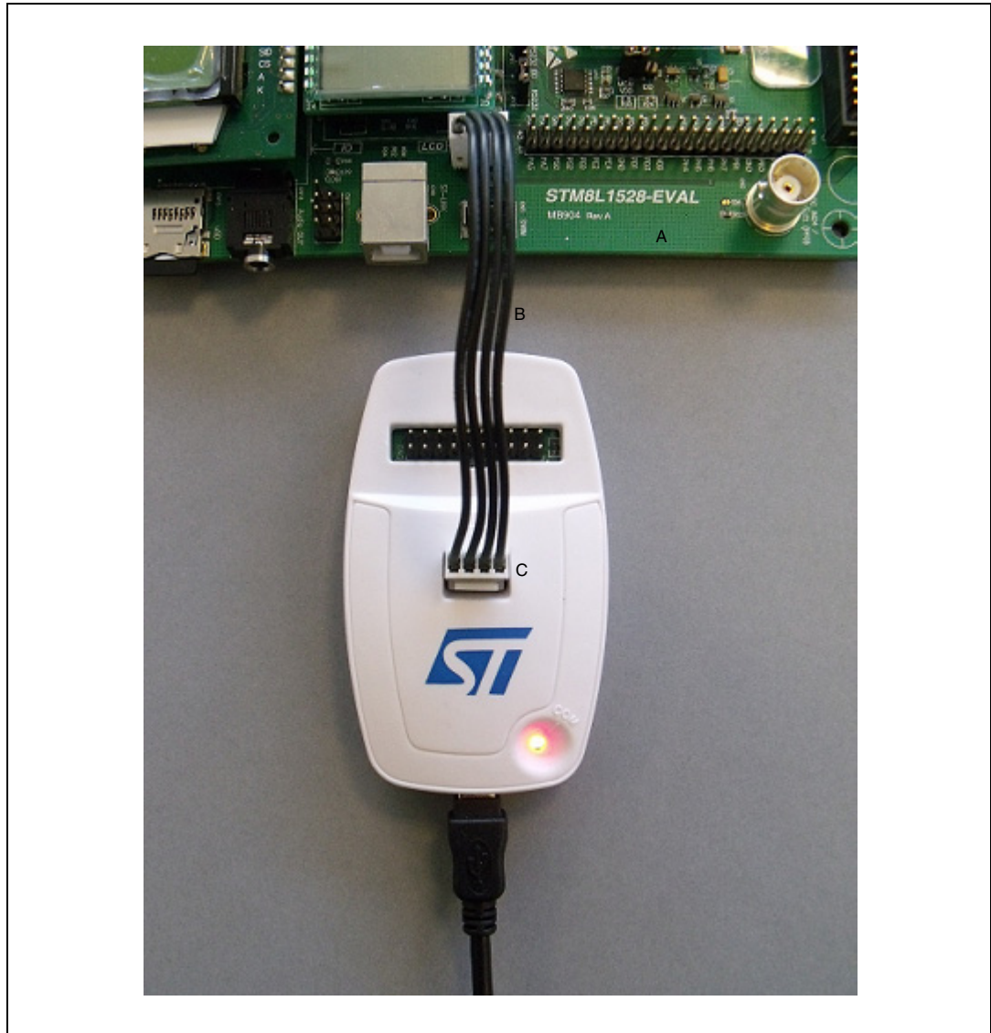
Figure 5. Low cost connection
